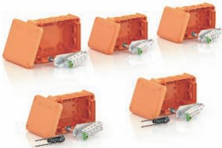
Halogen-free junction box with soft plug-in seals, including pre-mounted connection unit made of high temperature-resistant special ceramic and labelled protective conductor terminal. Supplied with 2 fire protection screw ties MMS 6x50 for anchorless fastening through the box bottom. High protection rating IP65, impact resistance class T100ED... IK08; T160ED... IK05.
