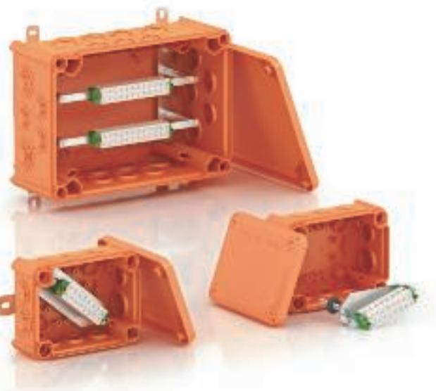
Halogen-free junction box with soft plug-in seals, including connection unit made of high temperature-resistant special ceramic and labelled protective conductor terminal for internal and external fastening. Supplied with 2 fire protection screw ties MMS 6x50 for anchorless fastening. High protection rating IP65, impact resistance class T100ED... IK08; T350ED... IK06.
