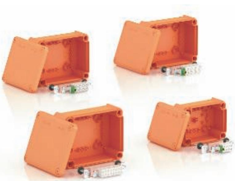
Halogen-free junction box, closed version, including pre-mounted connection unit made of high temperature-resistant special ceramic and labelled protective conductor terminal. Supplied with 2 fire protection screw ties MMS 6x50 for anchorless fastening through the box bottom. High protection rating IP65, impact resistance class T100ED... IK08; T160ED... IK05. Freely positionable cable outlets with V-TEC glands in the side walls.
