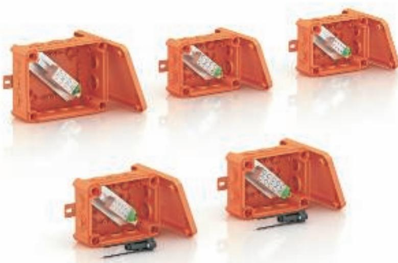
Halogen-free junction box with soft plug-in seals, including completely mounted connection unit made of high temperature-resistant special ceramic and labelled protective conductor terminal for external fastening. Supplied with 2 fire protection screw ties MMS 6x50 for anchorless fastening on the external shackles. High protection rating IP65, impact resistance class T100ED... IK08; T160ED... IK05.
